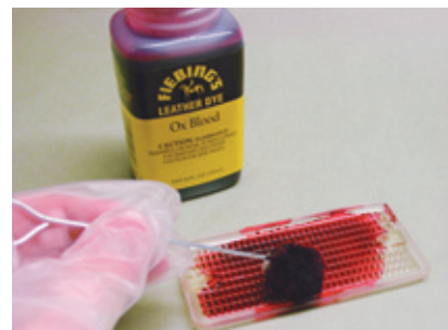
Figure 2: Apply aniline dye Aniline dye is applied to the model by brushing (shown), or dipping
