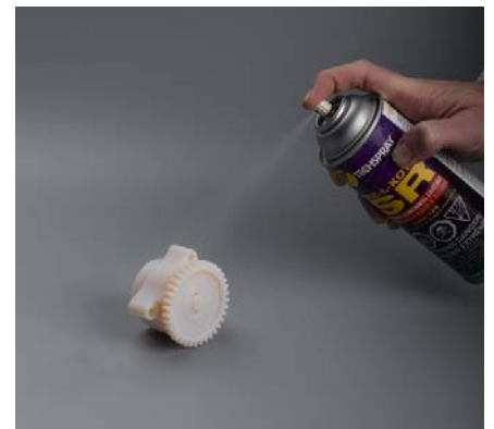
Figure 2. Applying chemical resistance spray on assembled parts
