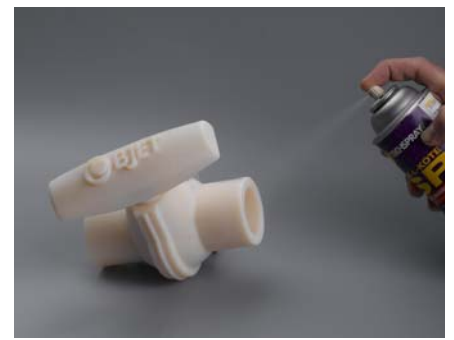
Figure 1. Applying chemical resistance spray
