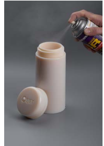
Figure 3. Coating the inner surface of the bottle
