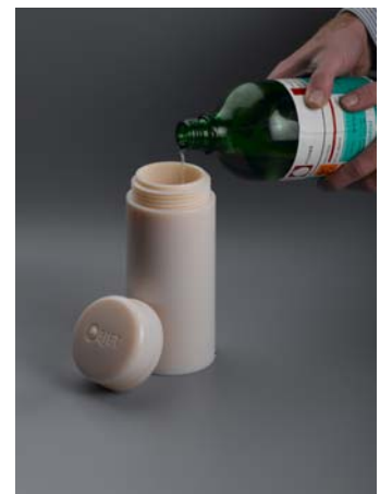
Figure 4. 72 hours later, the bottle is chemical resistant
