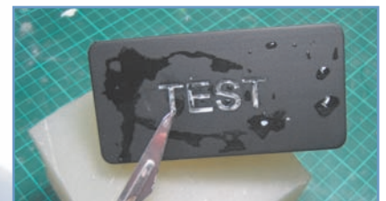
Step 6: Recessed Text – use scalpel or WaterJet
