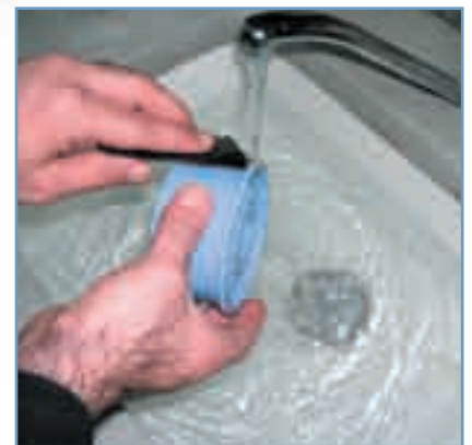
Figure 2. Wet-sanding. Wet-sand the model with 320-grid sandpaper.
