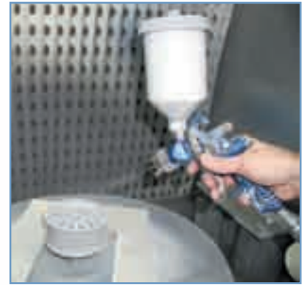
Figure 6. Apply Primer Paint.
