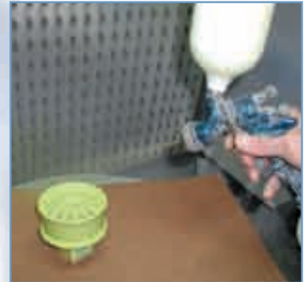
Figure 7. Apply Final Paint.
