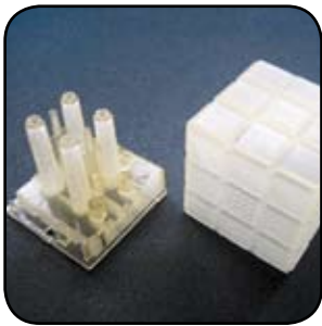
Figure 1: Prototype of an illuminated cube created on the Eden260™ Stylish Rubik's-Cube-shaped plug-in speaker flashes lights to music in your private space!
