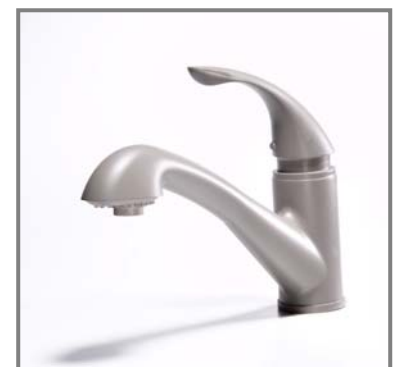
3. Metalizing the Objet model with a conductive surface
