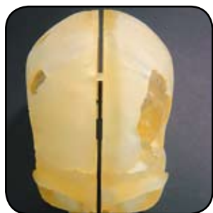
A printed replica fossil skull prepared for silicon moulding
