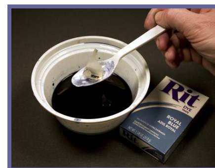
2. Soak part in warm water and powdered dye solution.
