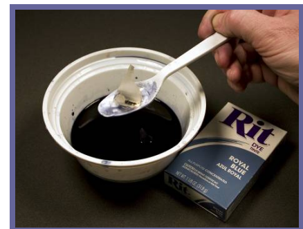
2. Soak part in warm water and powdered dye solution.
