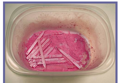
4. Dust parts in a container with powdered pigment.
