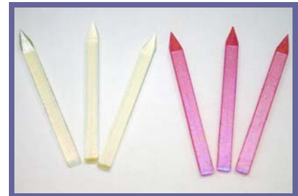
Clear needles printed in FullCure®720 (left) and dyed version (right).
