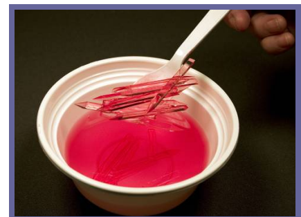
2. Soak parts in water and dye solution for approximately 15 minutes.
