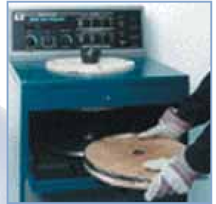
Figure 10: Placing the mold in the spin-caster
