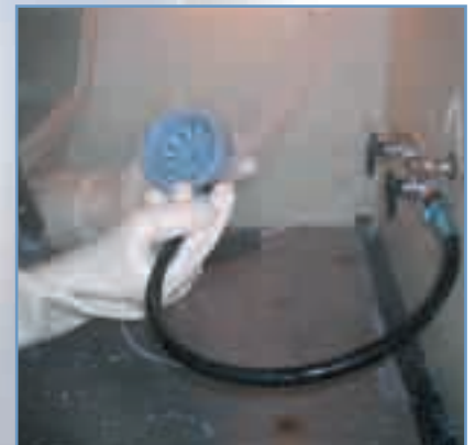
Figure 1. Removal of support material. Use WaterJet station to remove support material.
