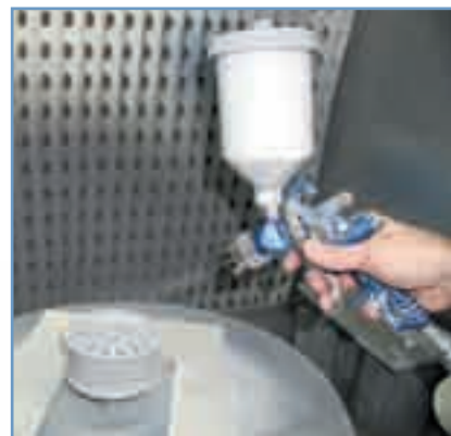
Figure 6. Apply Primer Paint.
