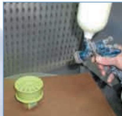
Figure 7. Apply Final Paint.
