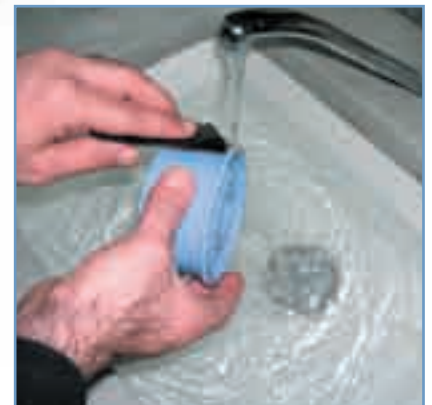
Figure 2. Wet-sanding. Wet-sand the model with 320-grid sandpaper.
