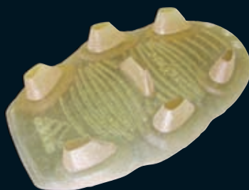
3-D Part with Support Structure Removed
