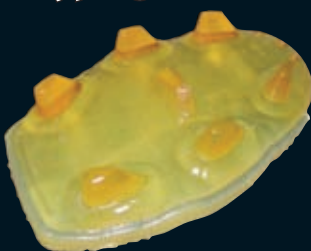
Objet Printed Part with Support Structure
