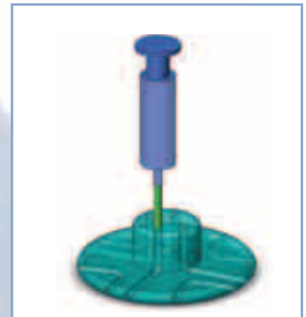
Figure 8: Injecting Proto-Reinforcement compound into printed mode
