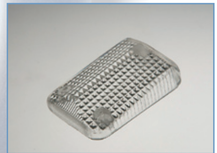
Figure 6. Finished model. The polished PolyJet model has the clarity needed for product demonstration.
