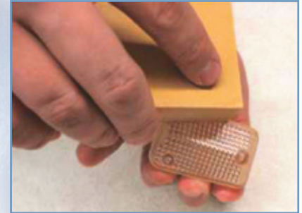
Figure 5. Micro-mesh sanding (optional). Using micro-mesh sandpaper, polish out all surface scratches prior to buffing.
