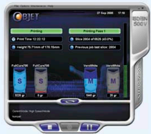
The System Display provides full visibility and control of the Eden printing system. It shows a progress bar, materials status indicators and printing time
