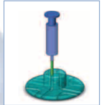
Figure 8: Injecting Proto-Reinforcement compound into printed mode
