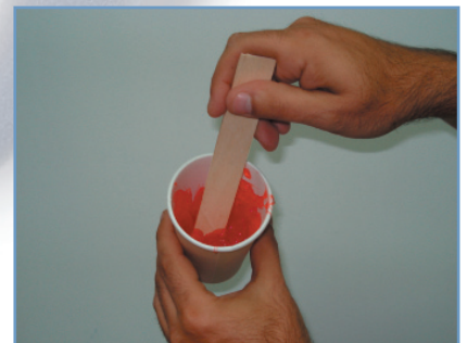
Figure 2. Preparing the silicone to be injected into mold.
