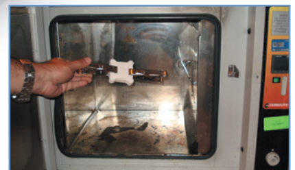
Figure 5. Mold is placed in oven for fast silicone curing.
