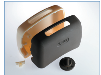
Picture 6. Ready model with RF shielding coating
