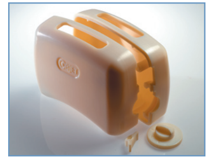
Picture 4. PolyJet™ part prior to coating
