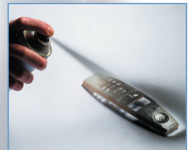
Picture 2. Applying coating onto PolyJet™ part
