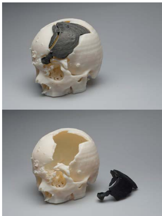
Fig 2. Medical models can be used to create prosthetic devices, such as implants precisely fabricated to match a cavity. Engineering features
