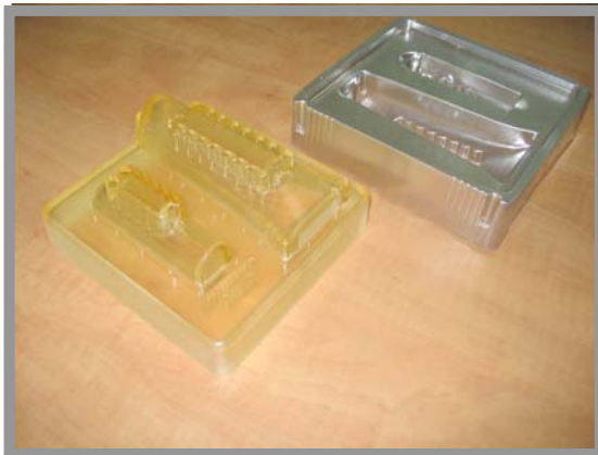
Figure 2: Printed 3D model using PolyJet Technology
