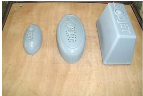
Figure 3: PolyJet models used in the vacuum-forming process
