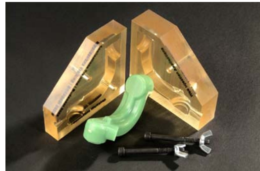
Figure 2: Printed PolyJet mold for wax injection
