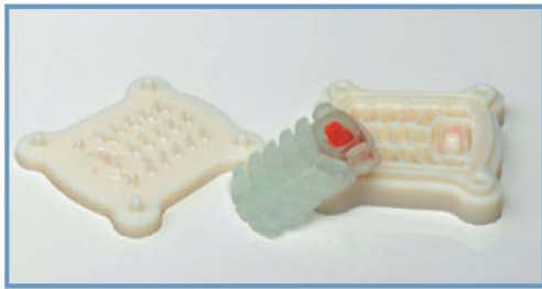
Figure 3: Printed mold for silicon injection
