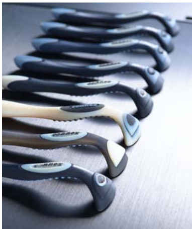
Image 2: All the razors in the image were printed simultaneously in a single run, within 12 hours. Every razor is composed of different materials (including Digital Materials) with different mechanical properties (rigid and flexible). These prototypes undergo feasibility tests and assist in defining the end-product's final materials
