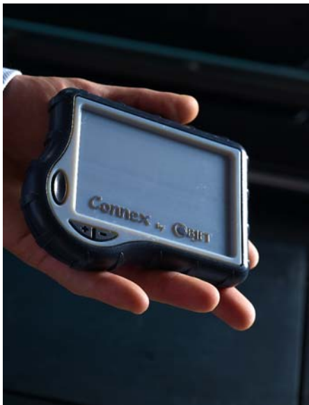
Image 4: A GPS device printed in a single run emphasizes an over-molded part. In this case, the rubber-like and rigid materials printed on the Connex500 at the same time eliminate the need for providing separate silicon molds of different materials and gluing them together, a process that normally takes several days to perform
