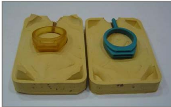
Figure 4: Rubber molds using PolyJet models
