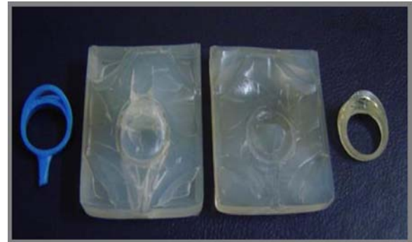
Figure 3: Silicon molds using PolyJet™ models
