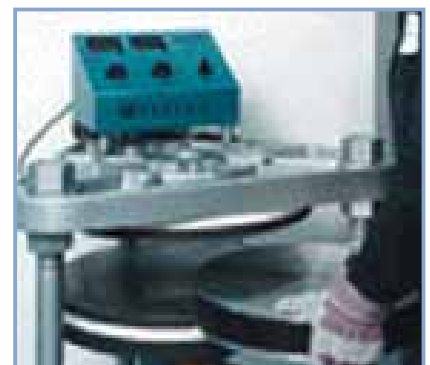
Figure 8: Vulcanizing the mold
